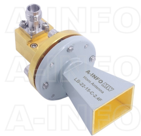
LB-22-15-C-2.4F Standard Gain Horn Antenna 33-50GHz 15dB Gain 2.4mm Female
